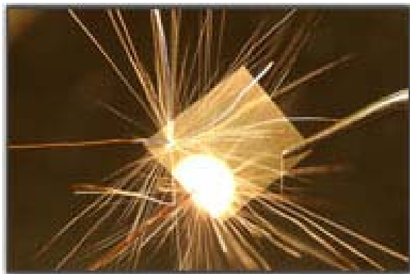
Reactive multilayer foil being ignited
