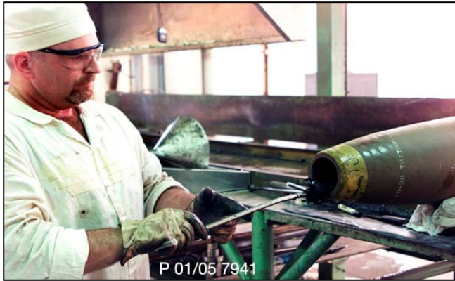
Remove Asphalt Liner
