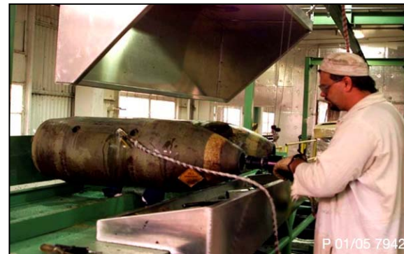
Cut Nose Fuze Well Conduit
