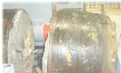
Steam Soften Asphalt Liner
