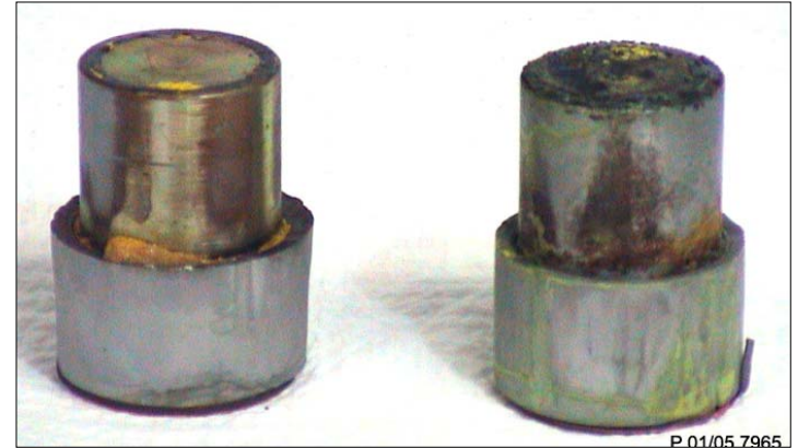
Fuzes cut out by Water Jet
