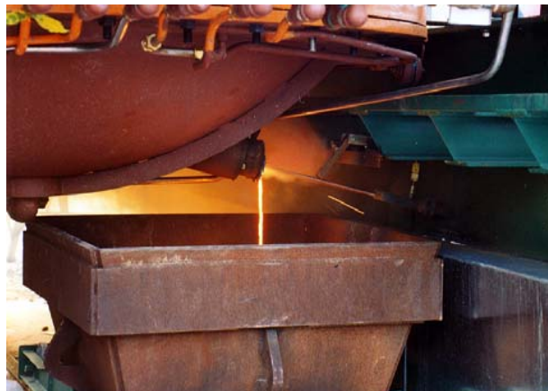
Plasma Arc thermal treatment system
