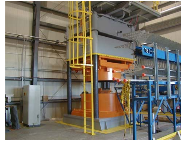
Munitions fractured in press
