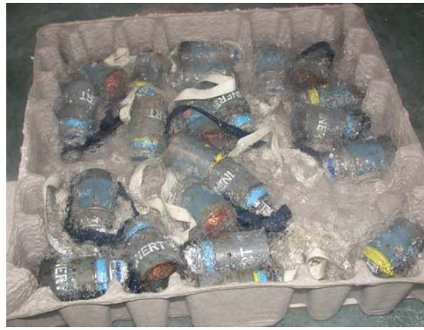
Munitions to be fractured in press
