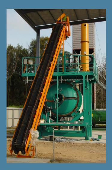
**UXB** International, USA, SDC2000 Delivered 2004. Installed in Asia Used for demil of AP and AT mines, projectiles, mortars, fuzes, detonators, grenades, bulk explosives and propellants, rockets HE, smoke, illumination, CS, WP
