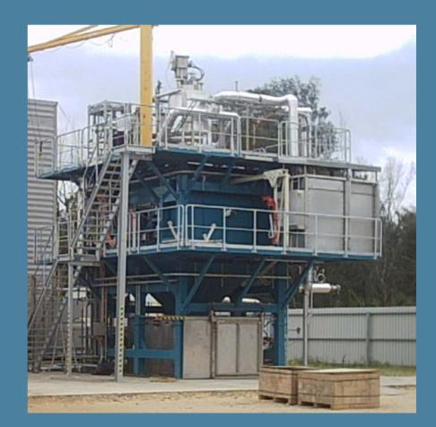
GEKA, Germany, **SDC2000** Delivered 2005 Used for demil of recovered Chemical Weapons, Airbags, conventional ammunition, bulk explosives and propellants Achieved 99.999999% DRE on HD (non-detect)
