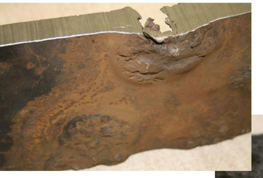
Cross section of protective floor plate 3' below sample
