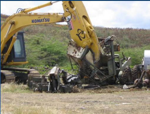
Downsizing target using the Shear
