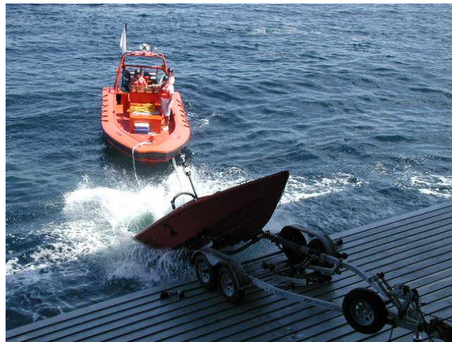
Launching a QST-33 SEPTAR off LPD 17's Stern Ramp
