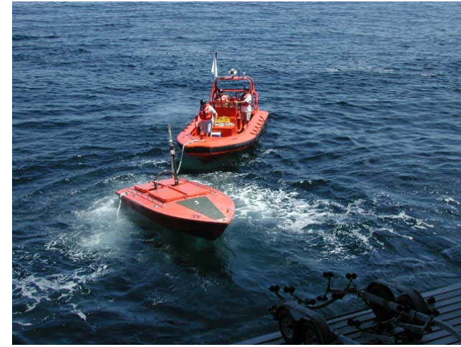
Launching a QST-33 SEPTAR off LPD 17's Stern Ramp
