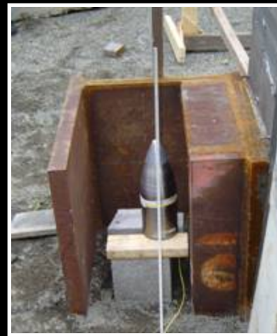
Fragment Velocity Test Setup
