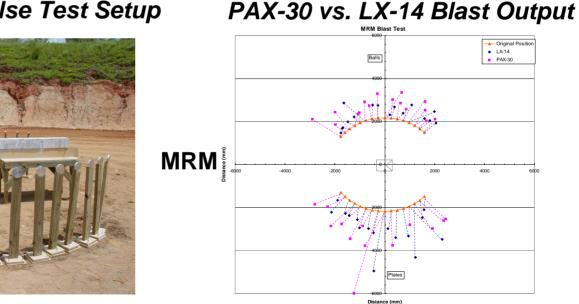
PAX-30 blast outperformed LX-14 in the MRM configuration.
