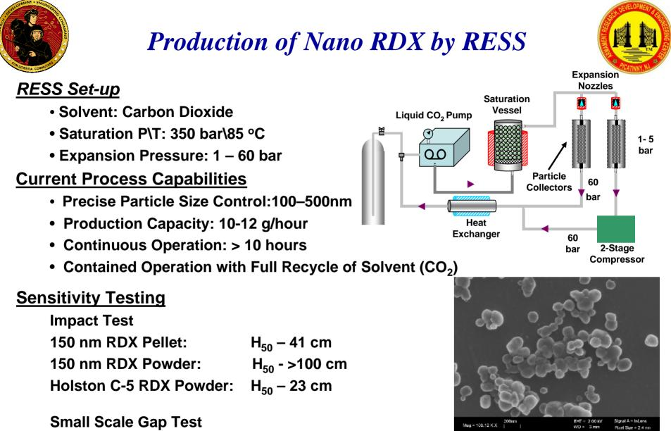
500 nm RDX in 88/12 wax formulation: Gap<sub>50</sub>- 32 kbar SEM Image of Nano RDX 4.8 micron RDX in 88/12 wax formulation: Gap<sub>50</sub>- 21 kbar
