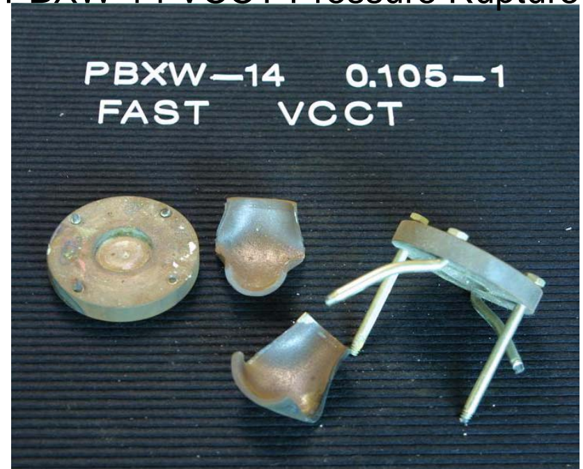
PBXW-14 VCCT Pressure Rupture
