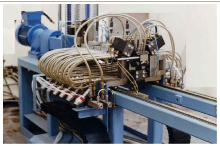
30 mm twin screw extruder to be installed in 2008
