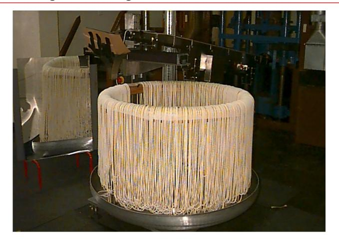
Propellant is draped and cut
