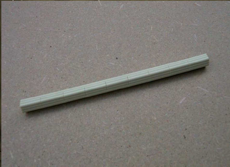
19-perf. kerfed rosette of GUDN-propellant.
