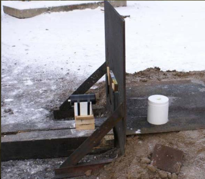
Spall impact test with UNIFLEX 2 IM and the FFV551 84 mm HEAT war head.
