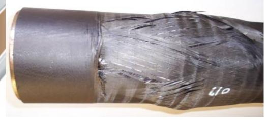
Hybrid laminate to reduce confinement of slender motors at elevated temperatures
