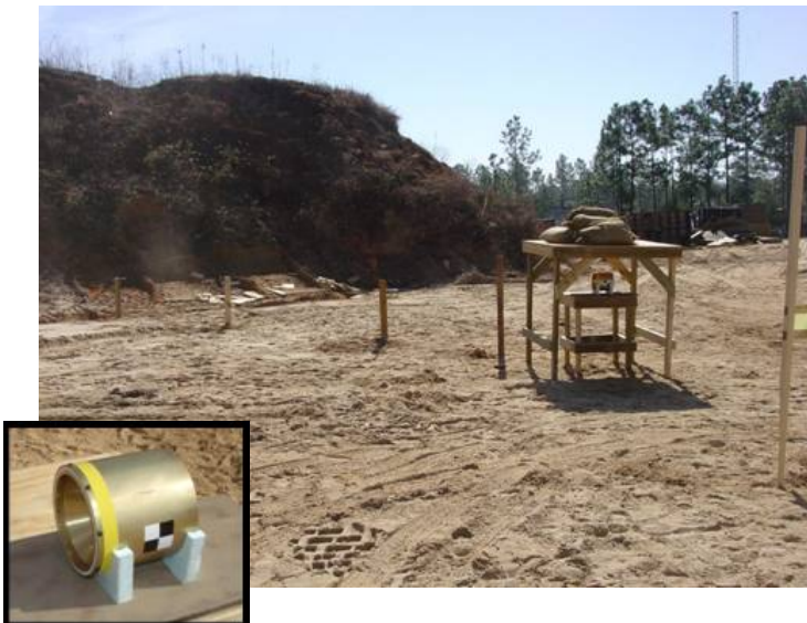
6000 ft/sec frag impact test setup
