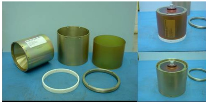
6000 ft/sec frag impact test setup
