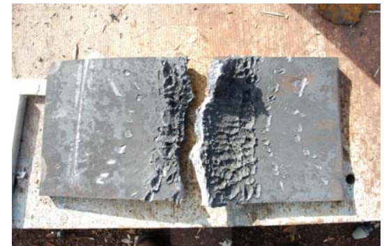
Witness plate after type 1 reaction
