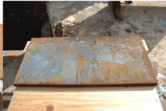
Witness plate after type 4 reaction
