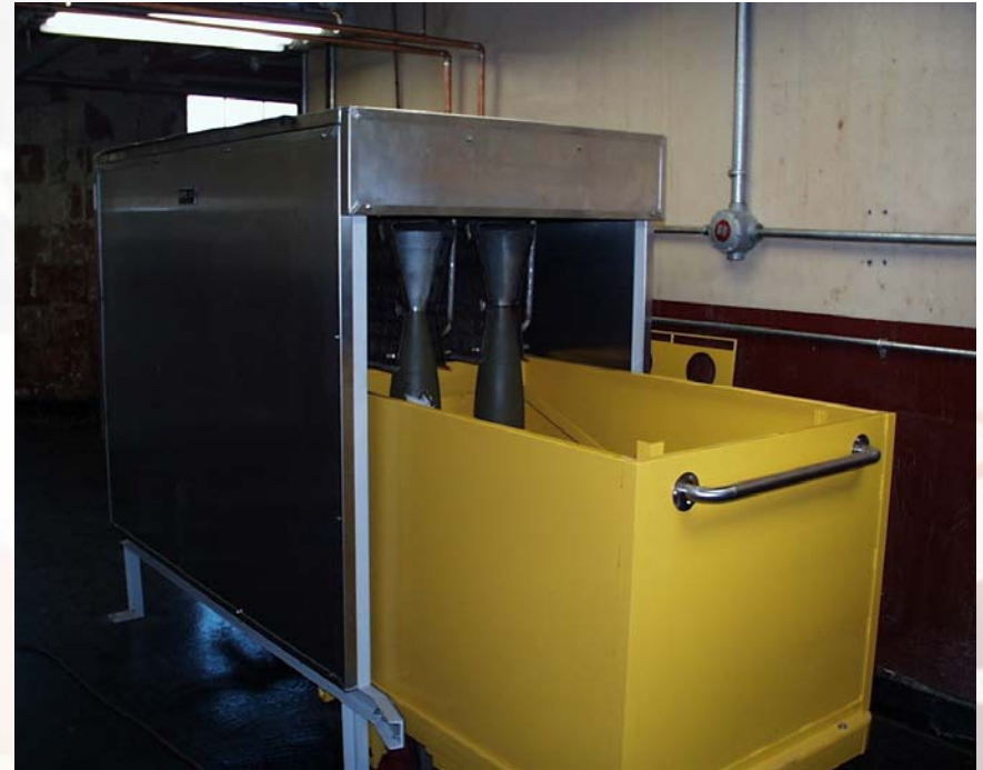
Controlled Cooling Oven
