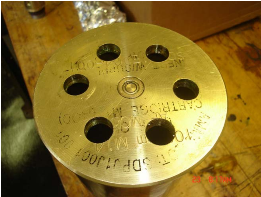
Cartridge case with 6, \frac{3}{4} inch holes
