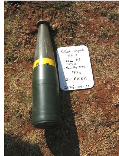
Explosive remains in shell above bullet track
