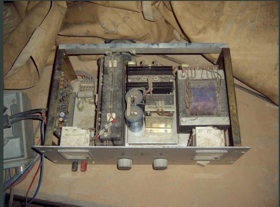
Actual operational power supply rigged by soldiers to run $500,000 thermal sight in theater
