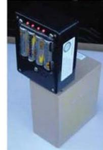
**MRC-41** – holds primary or rechargeable battery, powers the AN/PRC-148.
