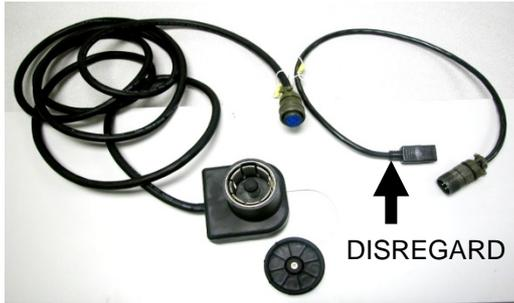
J-6362A/U DC slave cable for the PP-8498A/U (SPC). Disregard the smaller cable (attached), it is only used with the legacy PP-8444A/U.
