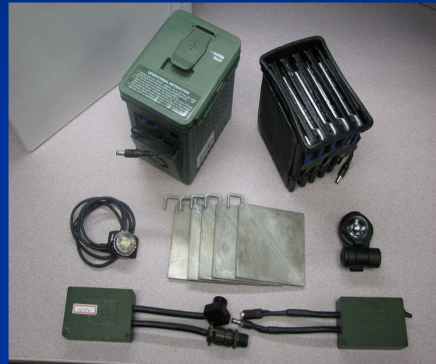
Metal Cell Batteries (Still under evaluation)
