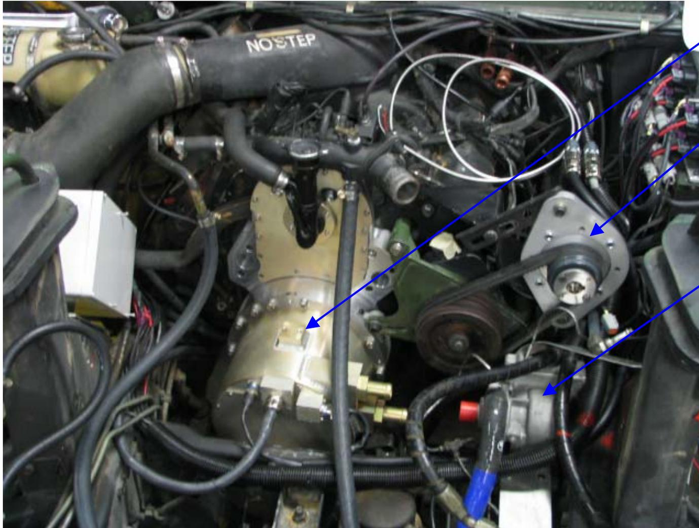
**ISG mounted on HMMWV engine crankshaft**
