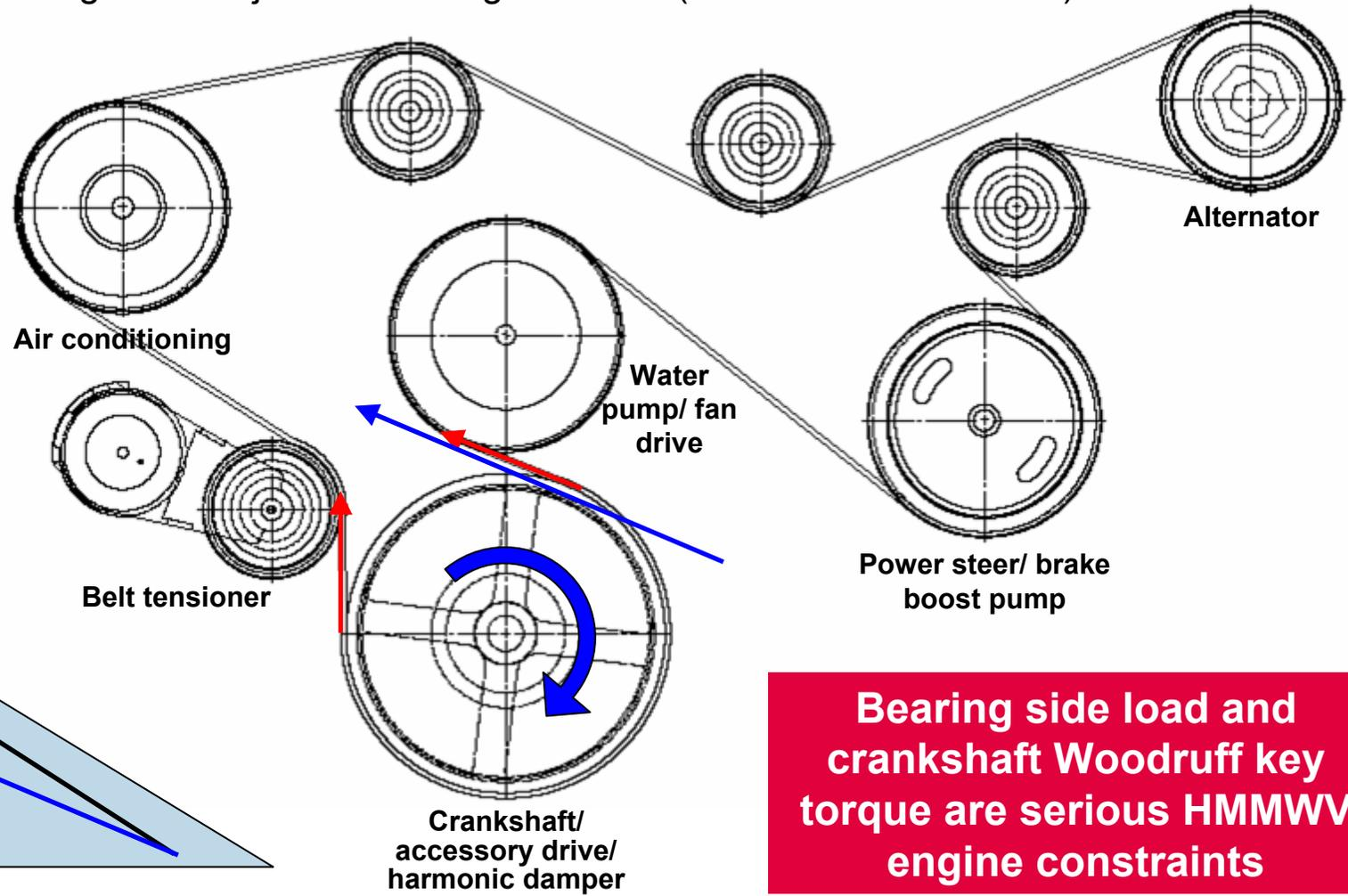
**Bearing side load and crankshaft Woodruff key torque are serious HMMWV engine constraints**
