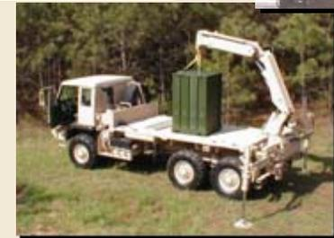
CLU Contains 15 Missiles, Battery, Fire Control and Communications System
