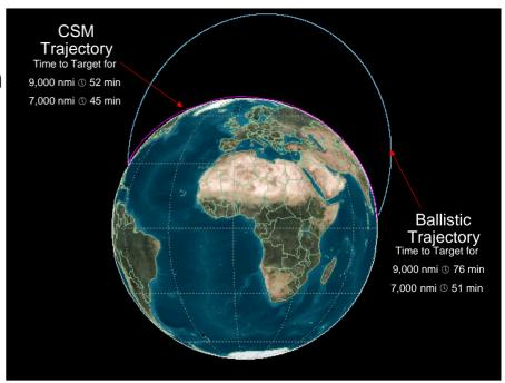
The HGV has a completely different profile and trajectory then a RV
