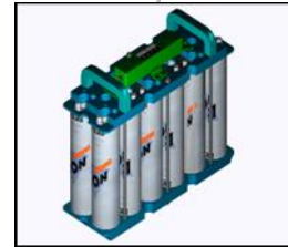
Li-Ion battery module w/ distributed DC/DC power converter
