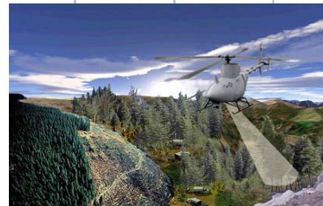
ARTEMIS - Foliage penetrating radar for CL IV UAV
