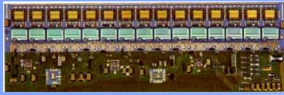
**240-channel multichip module for Si drift detector readout**
