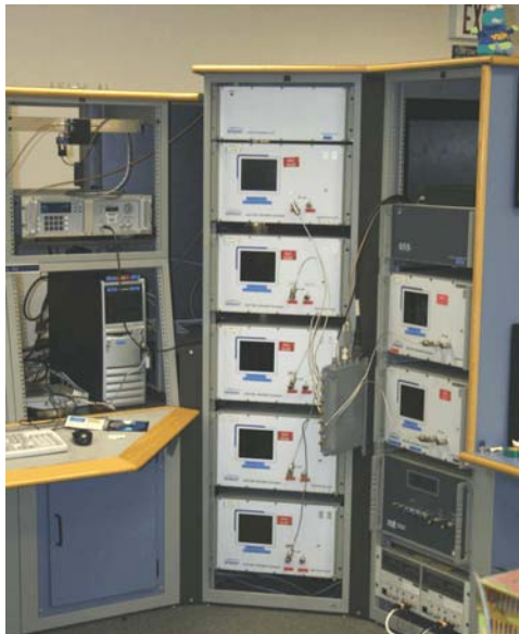
Coherent Wave Front Sim for GPS and Jamming signals
