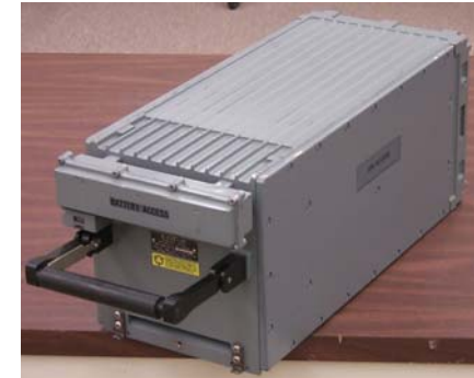
GPS: 5 Channel PPS Satellite Receiver
