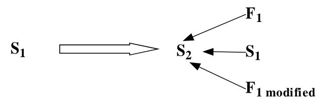
Example: To detect a moment when liquid starts to boil, an electrical current is passed through the liquid. During boiling, air bubbles are formed - they dramatically reduce electrical resistance of the liquid.
