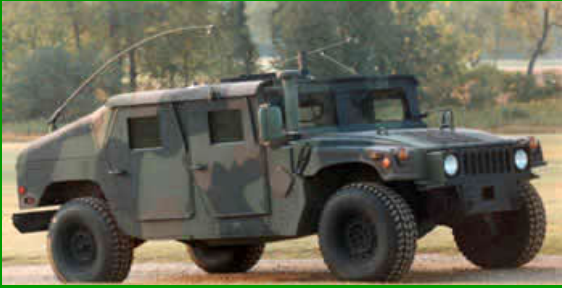
M998 HMMWV 4x4 High-Mobility Multipurpose Wheeled Vehicle
