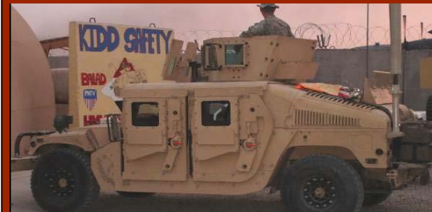
M1114 with the Objective Frag Kit 5
