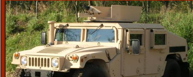
M1151A1 with the Objective Frag Kit 5
