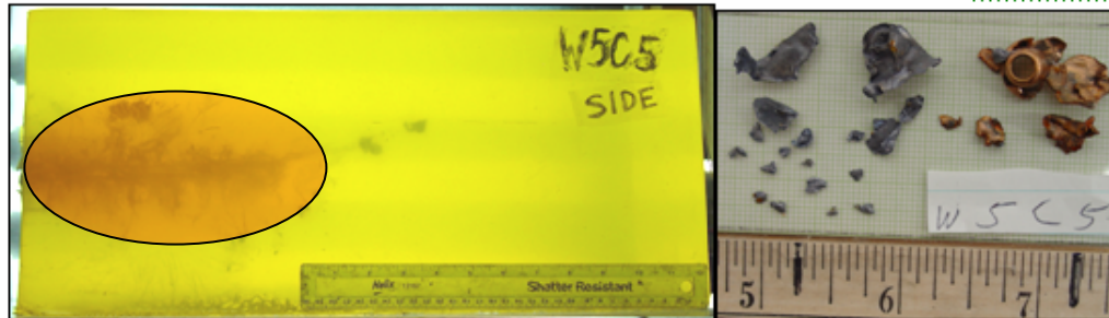
Figure 5. M855 vs. M80 through Auto Windshield
