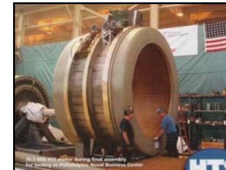
AMSC - 50,000 SHP (36.5MW) HTS AC Synchronous Motor
