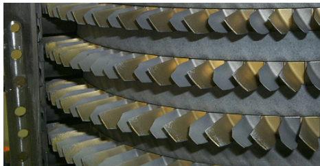
Russian erosion-resistant coating triples life of compressor blades in MH-53 helicopter, avoiding $1.6 million annually
