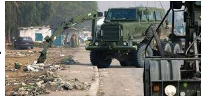
South-African developed Buffalo mine clearing vehicle probing & clearing mines & IEDs in Iraq
