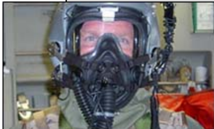
Joint Service Aircrew Mask Rotary Wing/Fixed Wing
