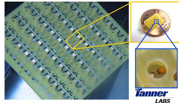
Micro-scale initiators on a PC-board substrate
