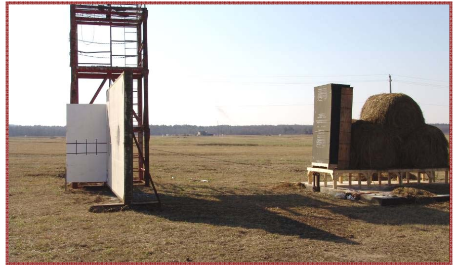
DRC Target Wall and Celotex/Hay Soft Catch
