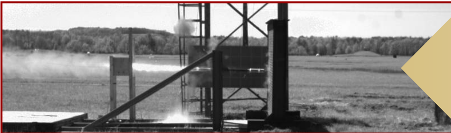
SMF Round in free-flight into Brick-over-Block (BoB) Wall
