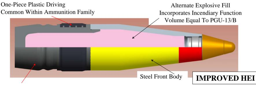
Aft Body Is Cobalt Free Tungsten Alloy With High Iron Concentration Boattail Added For Reduced Drag, Same As PGU-14/B API
