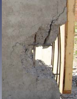
8" Double Reinforced Concrete
