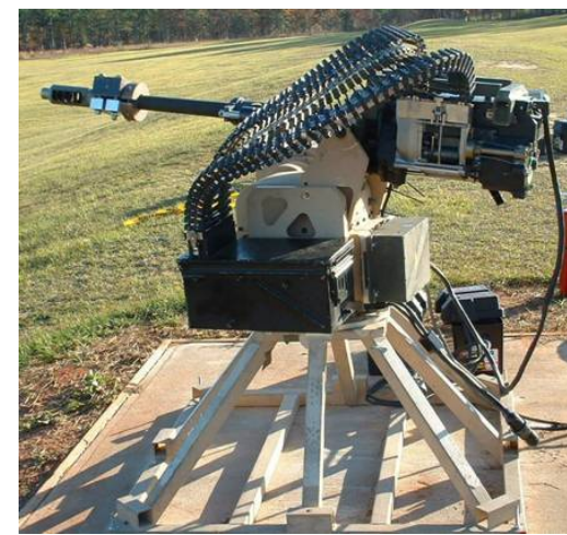
Recon Optical's RAVEN R-400 is used for common remotely operated weapon station (CROWS) program.
