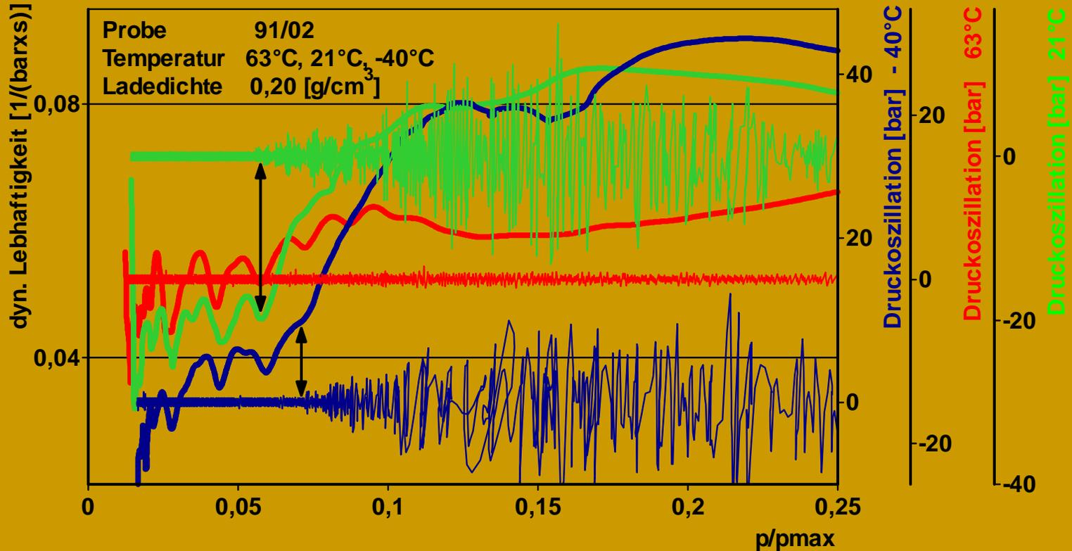
**At +63°C: only weak oscillations - regular behaviour of the dynamic vivacity**
