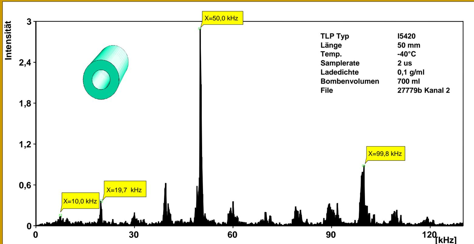
Characteristic maxima of frequencies associated with the fundamental frequency (10 kHz)
