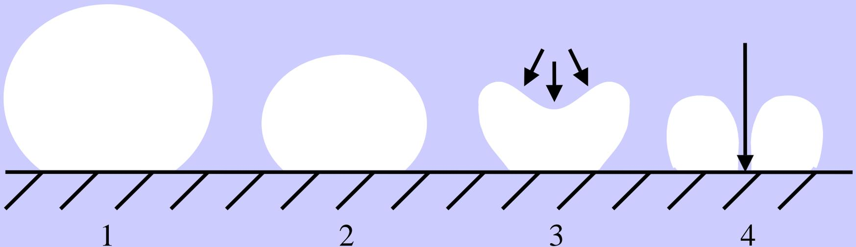
Cavitation bubble imploding close to a fixed surface generating a jet (4) of the surrounding liquid.
