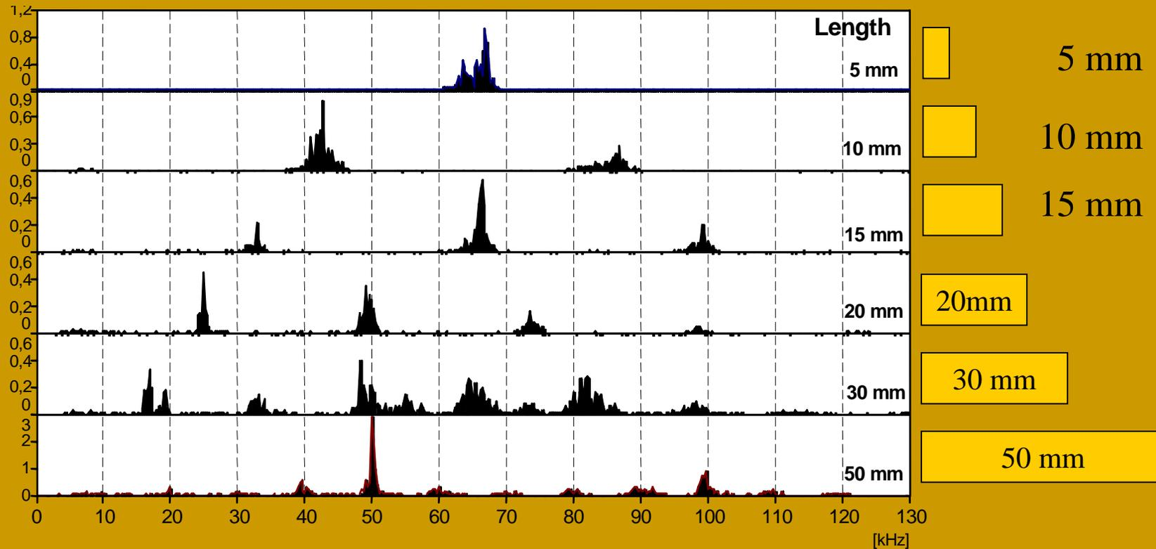
The shift of the frequencies proves that the oscillations are connected with the tube lengths.
