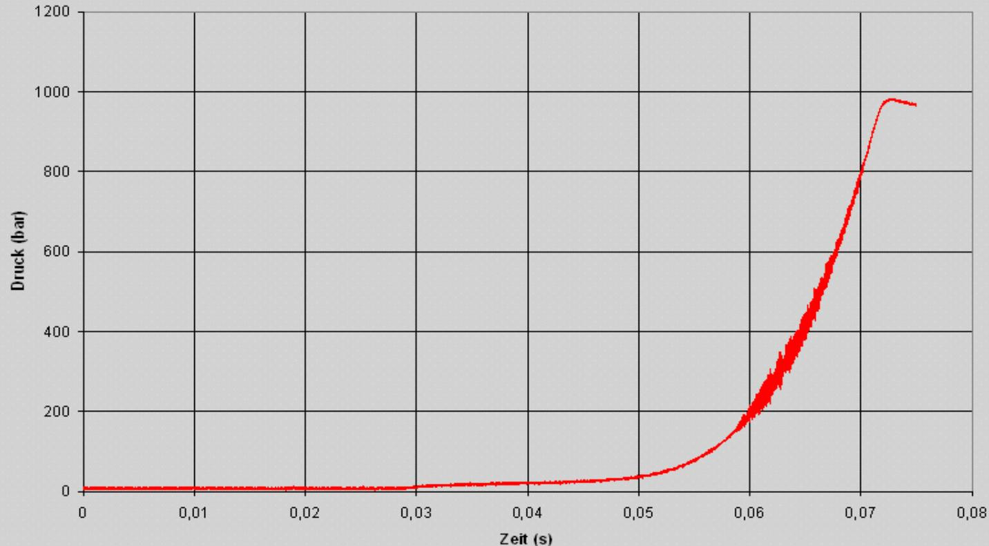
Confirmation of the existence of pressure oscillations when burning propellant grains
