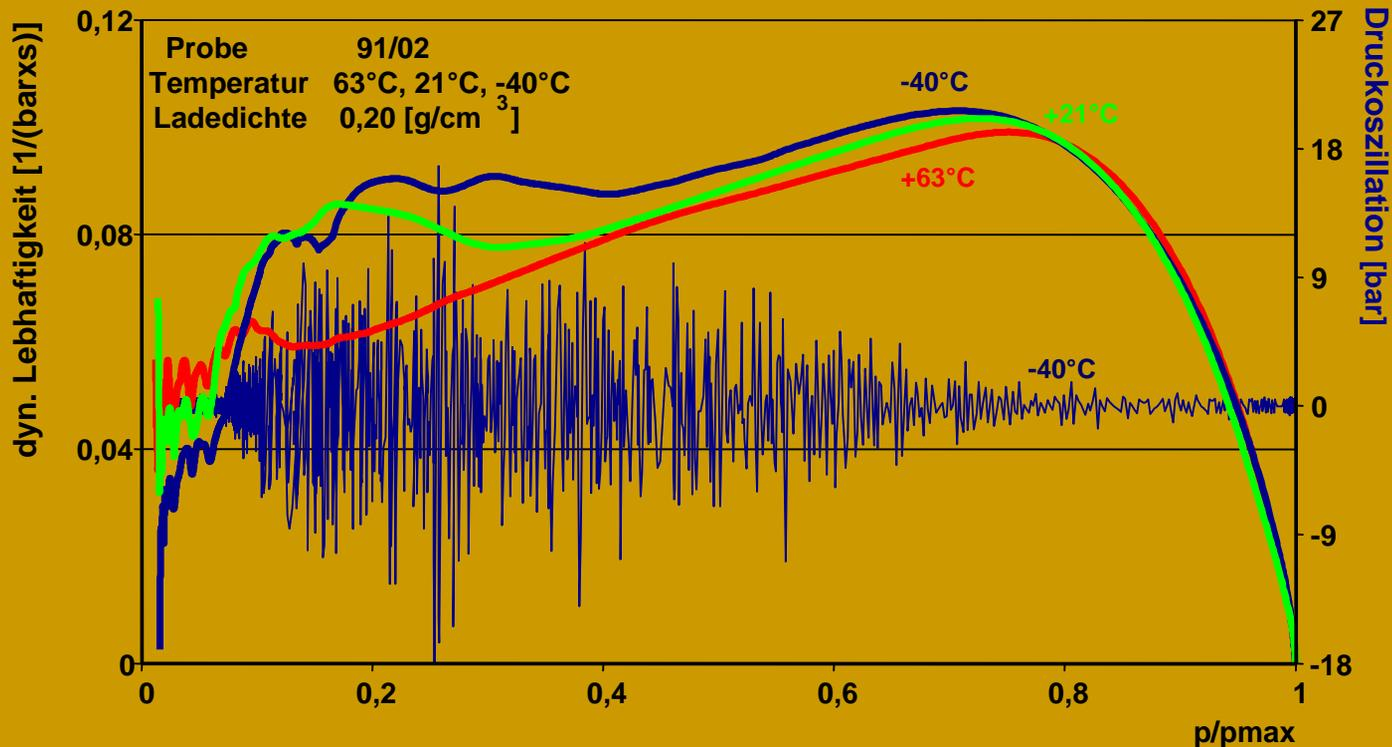
Reversal of the temperature behaviour for the perforated propellant within the temperature range from +63 (+145°F) to - 40°C (- 40°F). The vivacity of the perforated propellant increases with temperature. The excessive burning corresponds with the intensity of pressure oscillations.
