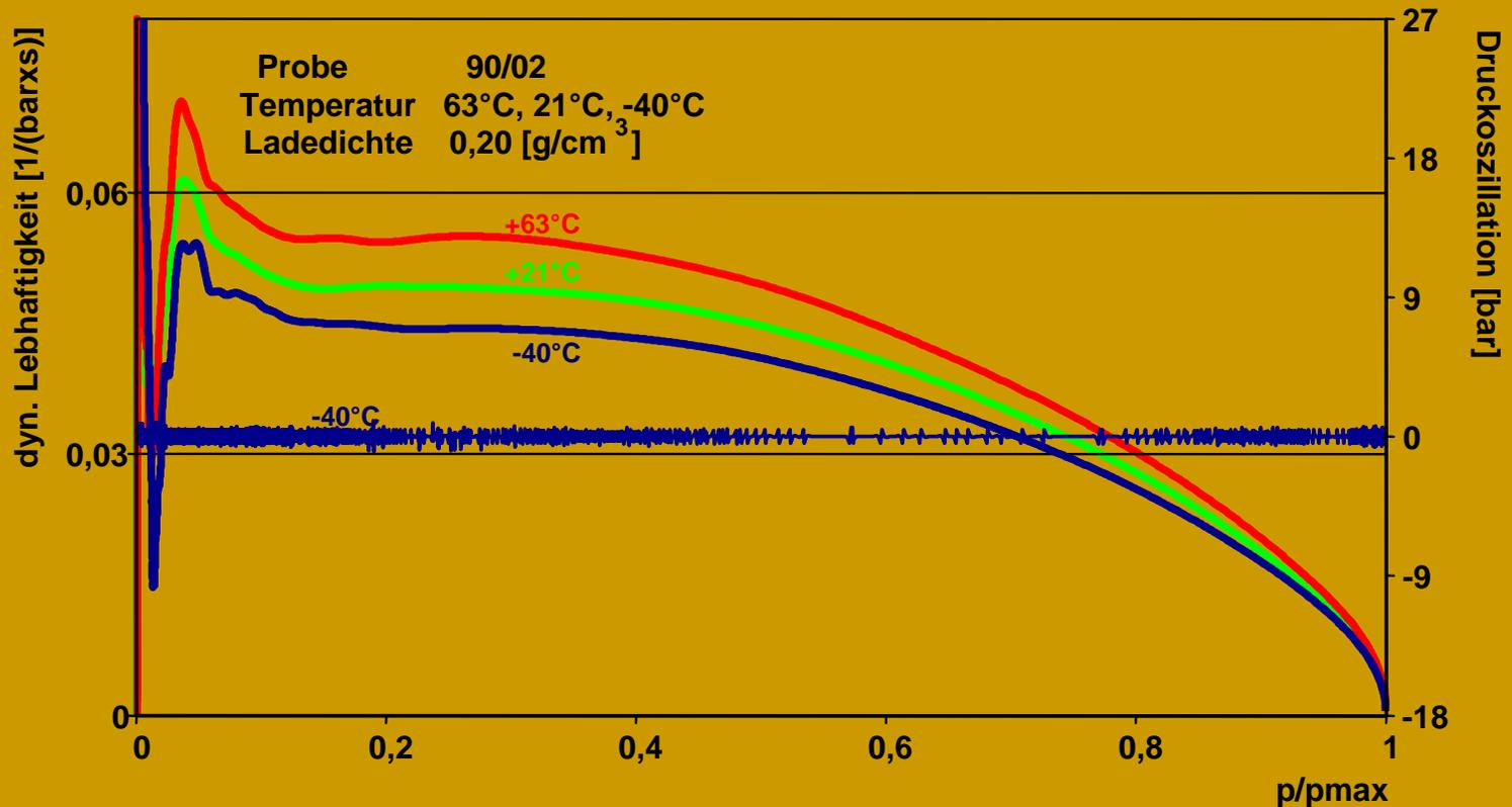
From +63 (+145°F) to -40°C (-40°F) the vivacity of the non-perforated propellant decreases with temperature. No noteworthy oscillations can be observed.
