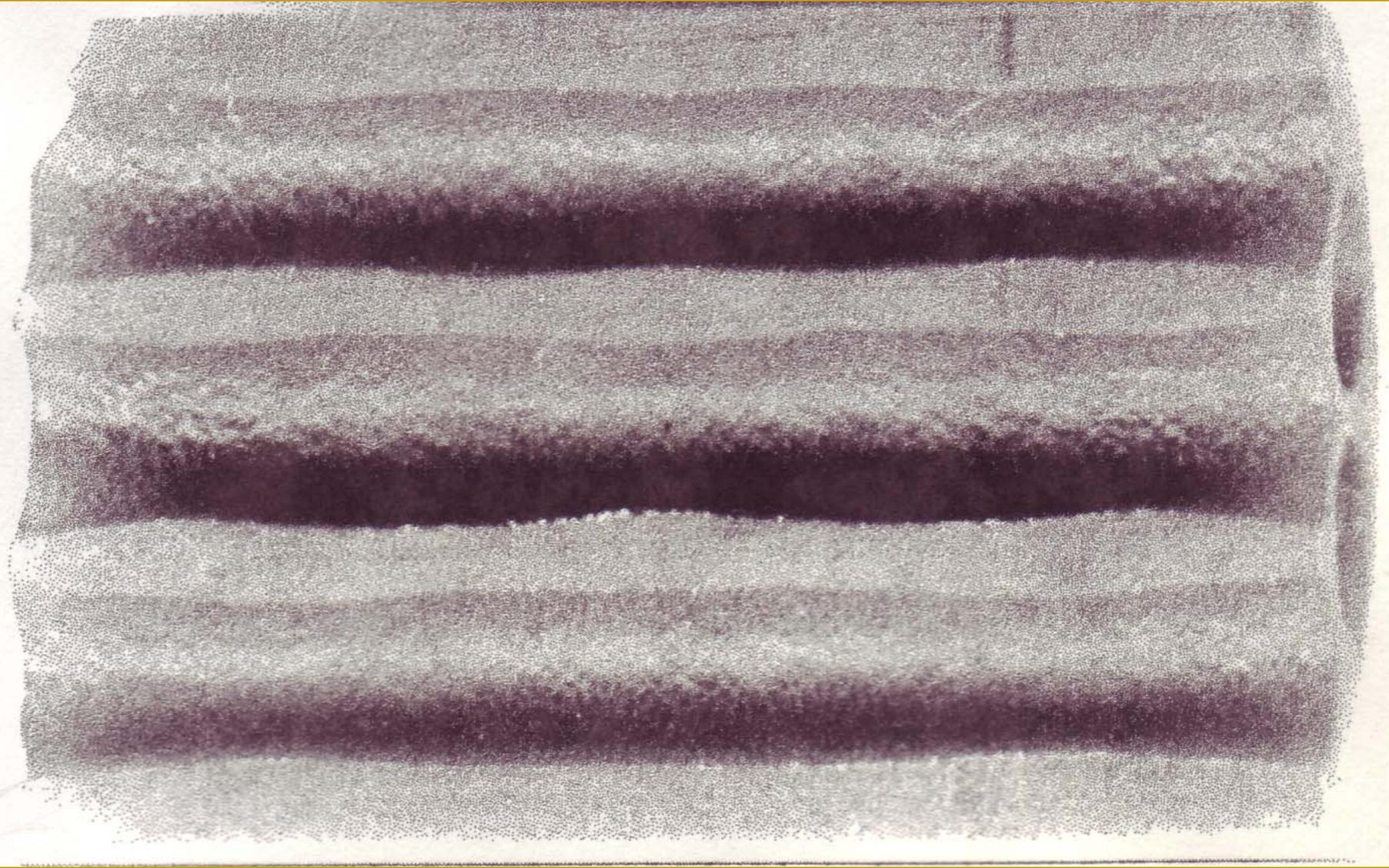
Double-base 7-hole-propellant grain after interrupted burning at  $-40^{\circ}\text{C}$  ( $-40^{\circ}\text{F}$ ).
