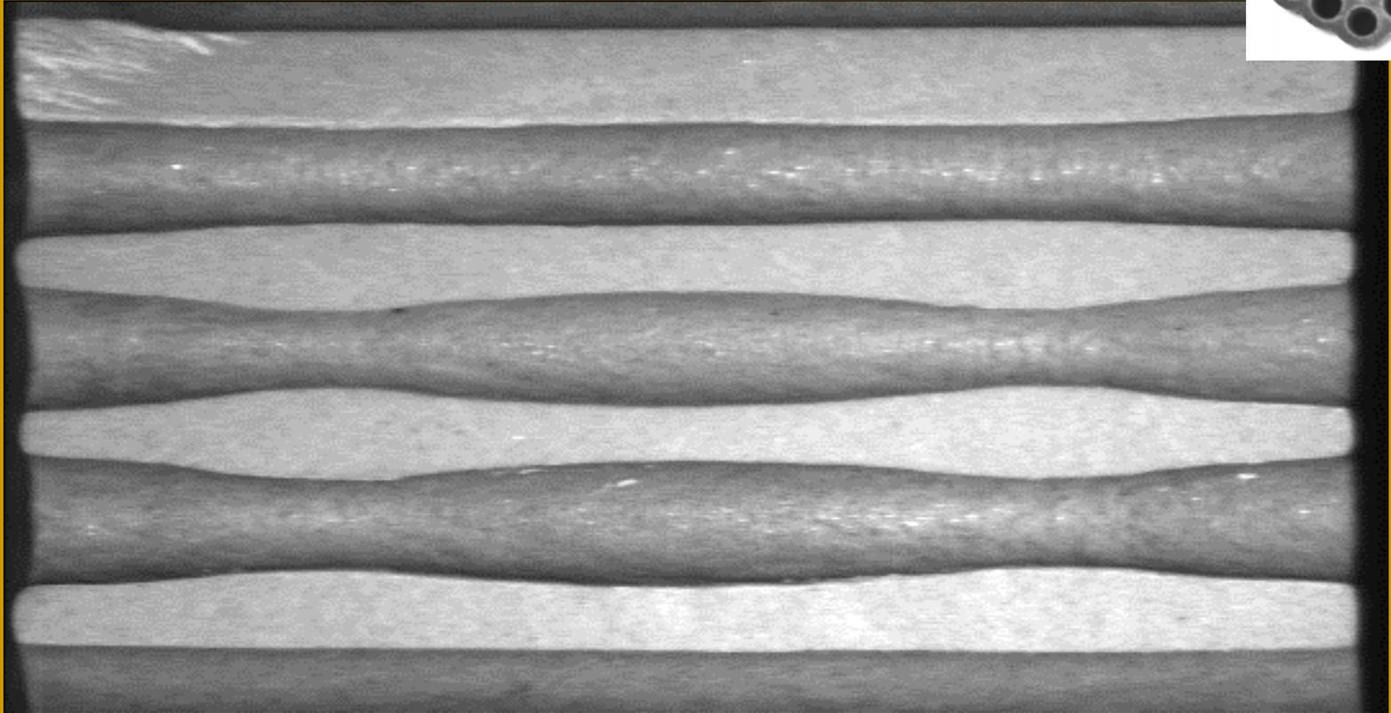
The picture shows a sectional view of a triple-base 19-hole-propellant grain after interrupted burning at  $-46^{\circ}\text{C}$  ( $-51^{\circ}\text{F}$ ). The wavelike erosions indicate the occurrence of standing waves in the holes.
