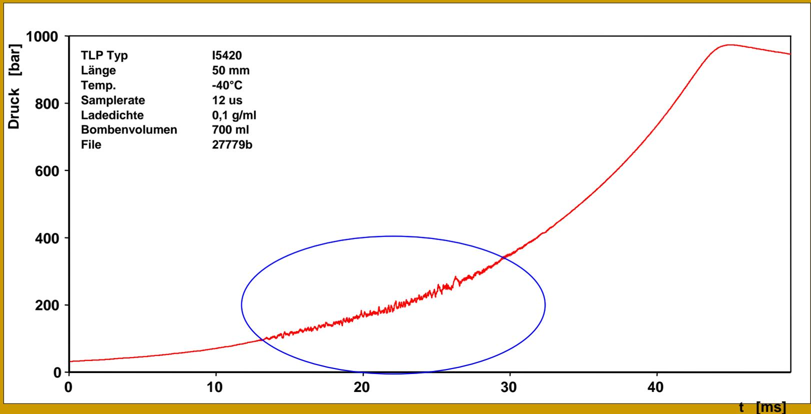
Pressure / time curve resulting from burning a tube propellant in a closed vessel.
