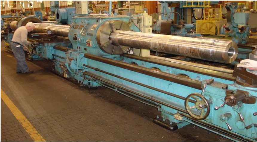
First Production Barrel on Hollow Spindle Lathe
