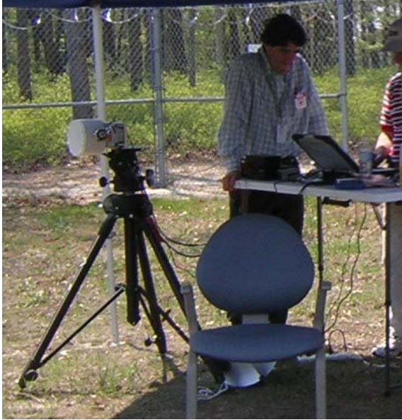
PPT Personnel Tracker Modified COTS Radar
