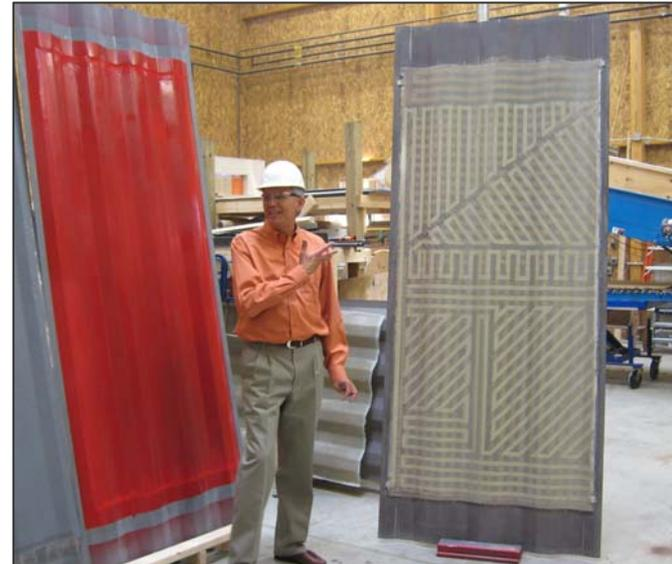
**Composite Material with Embedded Sensors**
