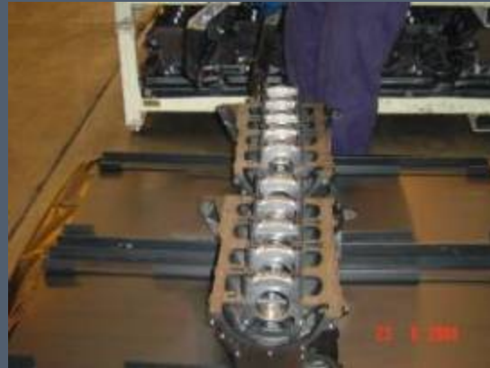
3) Blocks head bank down on Corex strips
