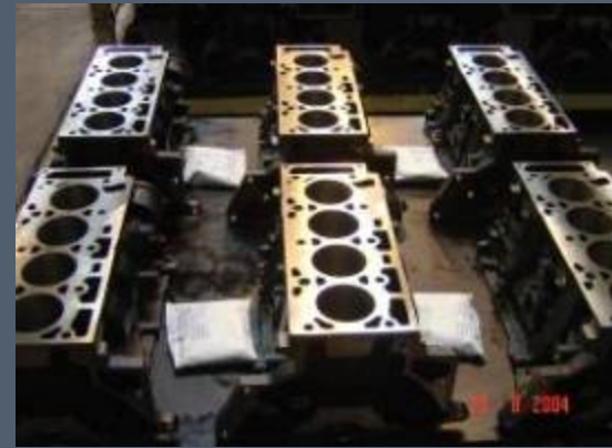
6) Blocks head bank up making 2 nd layer. Desiccants added as per # 4
