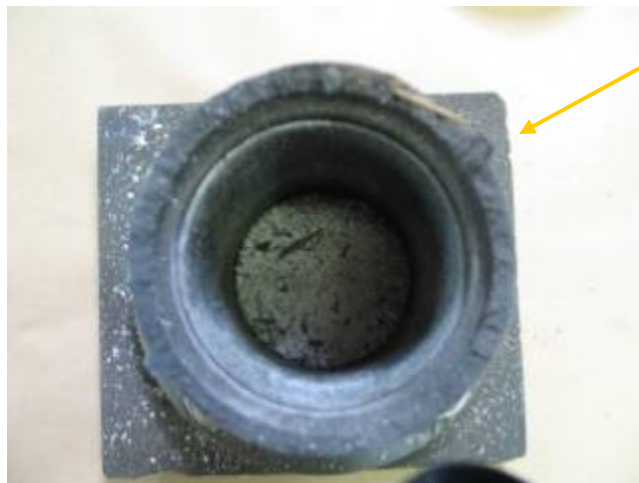
Top view of post test "pipe bomb" with minimal ANFO residue on bottom plate
