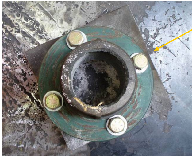
Top view of post test "pipe bomb" with minimal ANFO residue on bottom plate
