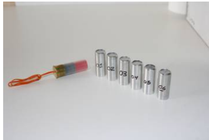
Disruptor round with inert slug for loading curves at top and rounds with APEX 17/17 RM at left
