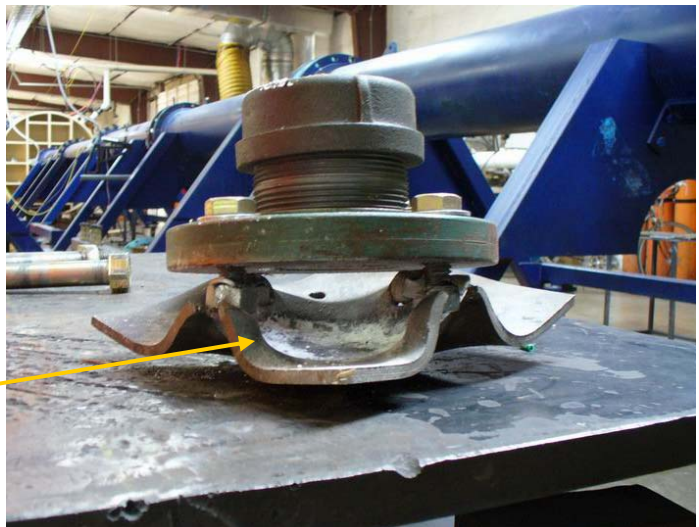
Top view of post test "pipe bomb" with minimal ANFO residue on bottom plate
