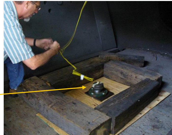
Test article loaded into explosion tank
