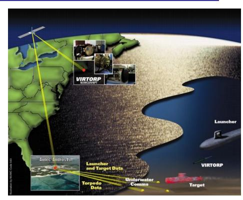
Naval Undersea Warfare Center Newport Synthetic Environment Tactical Integration Virtual Torpedo Project HLA federation linking live submarines to high-fidelity torpedo hardware-in-the-loop facility
