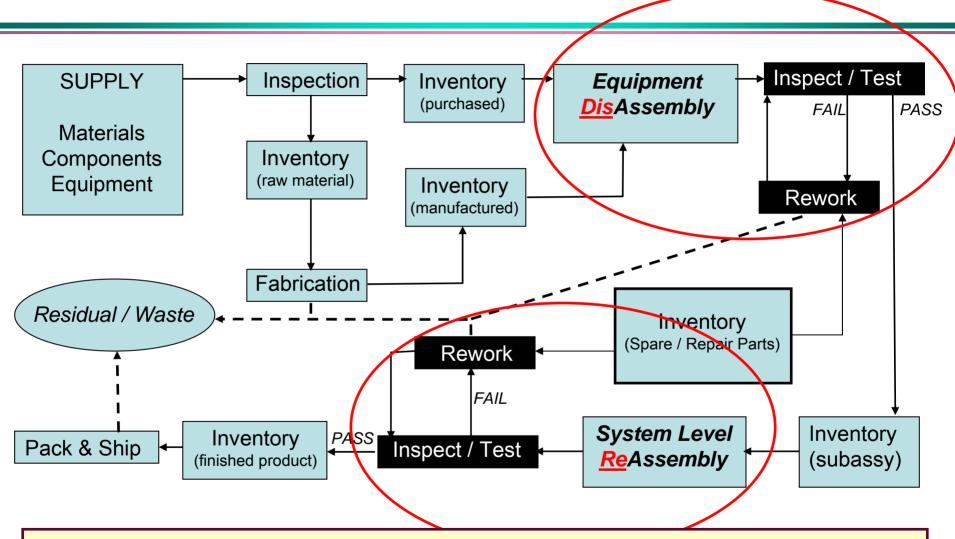
Maintenance concept & contractual stipulations for warranty repair may direct return of entire system or sub-assemblies for depot level repair
