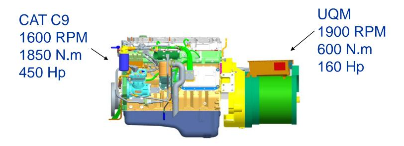
Combined Peak Torque 2446 N-m (1804 ft-lbf) @ 1600 RPM Combined Peak Power 610 HP (455 kW) @ 2300 RPM Four, 45A\*h
