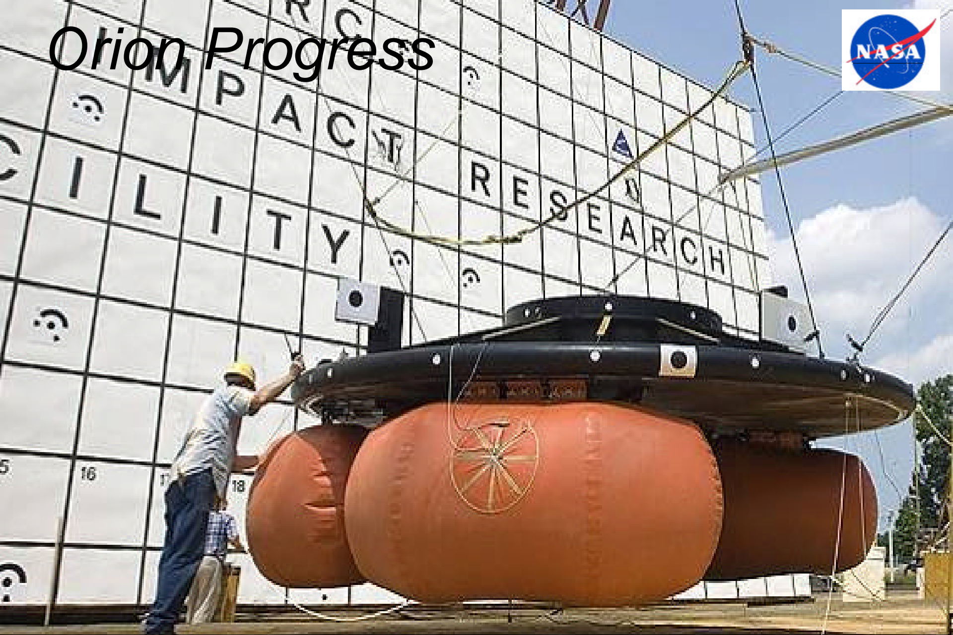
Landing System Airbag Tests
