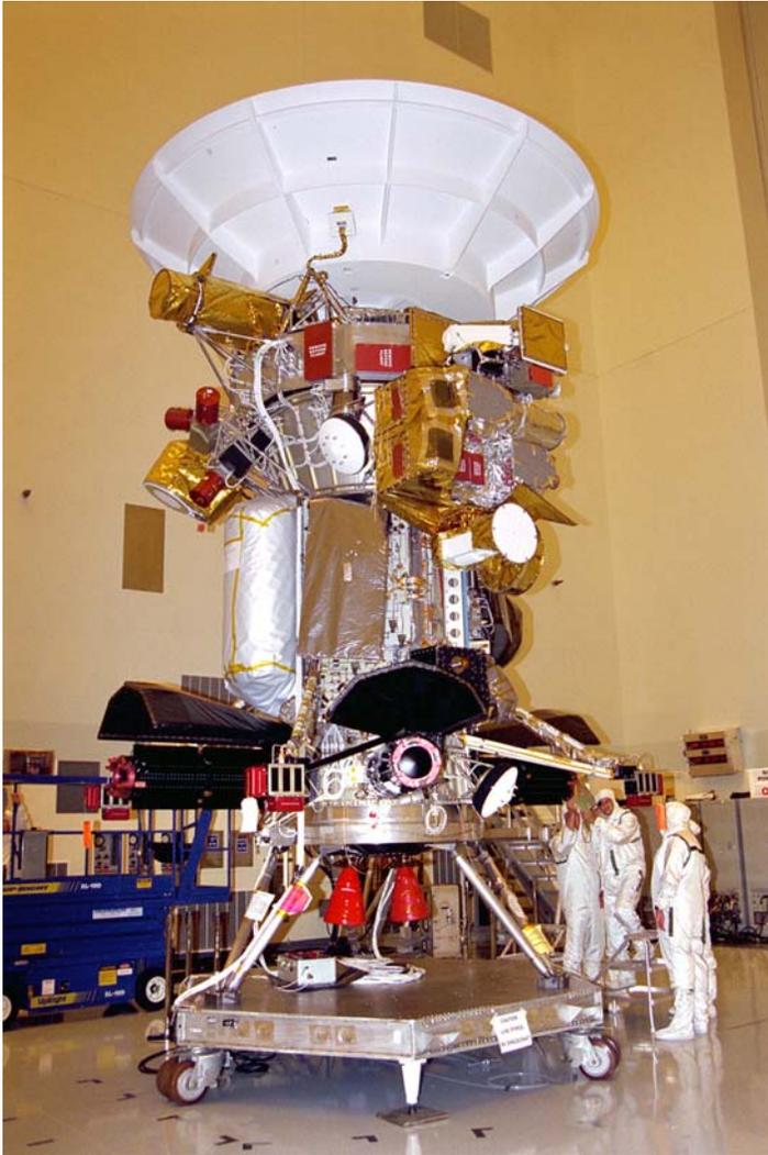
**SFM** was used in many cases to help understand complex system interactions and create isolation systems for the Huygens Probe
