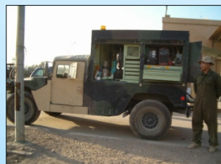
Rock Island Arsenal – Joint Manufacturing & Technology Center Shop Equipment Contact Maintenance (SECM)
