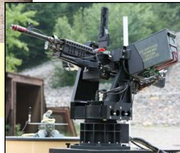
Picatinny Lightweight Remote Weapon Station (PLRWS) on TARDEC Advanced Robotic Platforms
